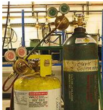
Fig. 1-3 A portable welding outfit, with oxygen and acetylene cylinders chained to an easy-rolling cylinder truck. Cutting attachment, normally a part of such an outfit, is not shown
