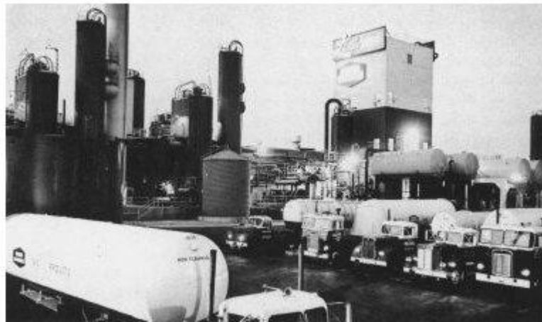
Fig. 1-1 A major oxygen plant, from which both liquid oxygen and liquid nitrogen are shipped by tank trailers to use points and cylinder filling stations which may be hundreds of miles away.
