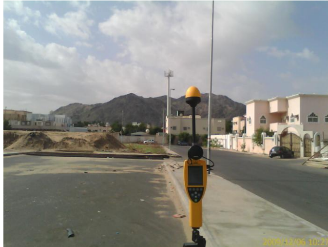
Fig.2: The Narda Broadband Field Meter. The picture was taken while performing the RF measurements at Al Awali site in Makkah.
