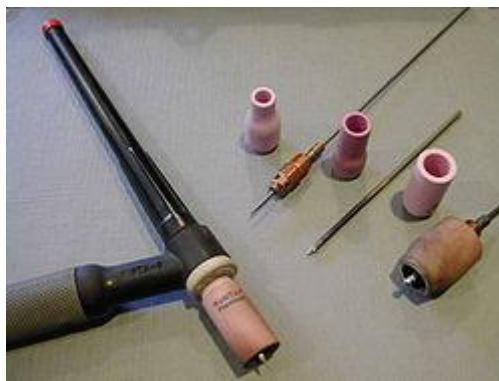
Figure 3-3 : GTAW torch with various electrodes, cups, collets and gas diffusers
