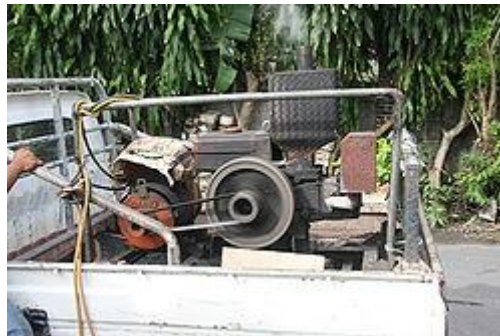
Figure 3-1 :A diesel powered welding generator (the electric generator is on the left) as used in Indonesia .
