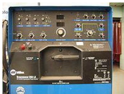
Figure 3-5 : GTAW power supply
