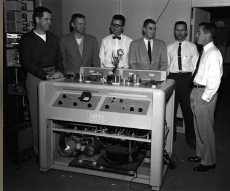
1956: Ampex VRX-1000 The First Commercial Videotape Recorder
