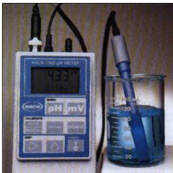
Fig. (9-2) : A pH meter uses the voltage of a cell to measure the H^+ concentration in a solution. Each change of one pH unit causes a voltage change of 0.0592 volts.
